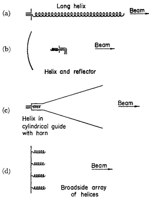
Fig. 8—High-gain antenna systems using helical beam antennas.
